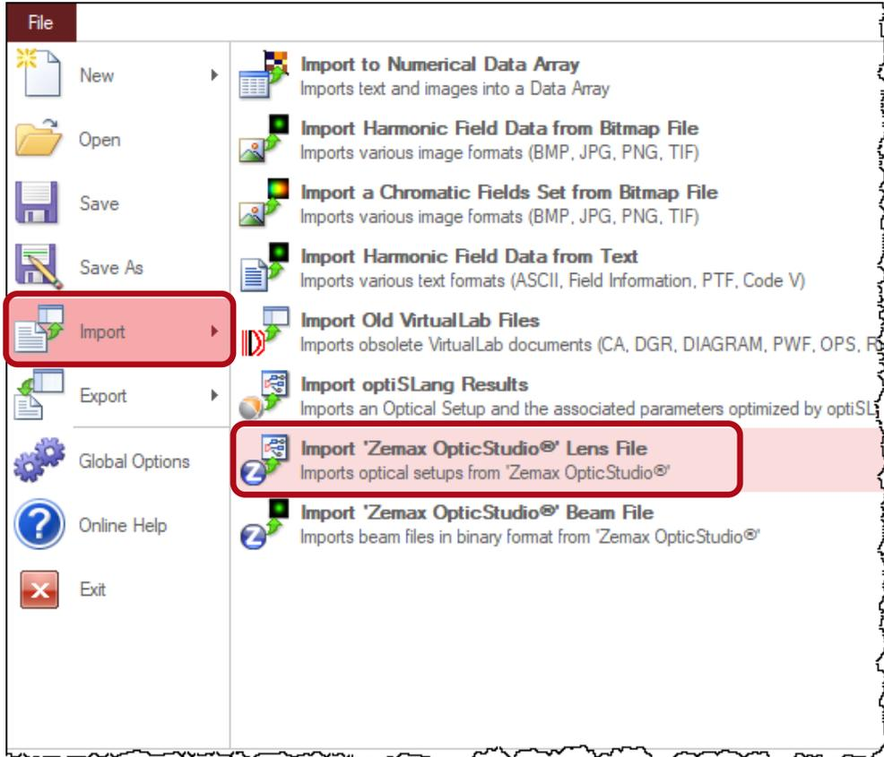
In VirtualLab Fusion, Zemax OpticStudio® files can be imported via the following steps:
