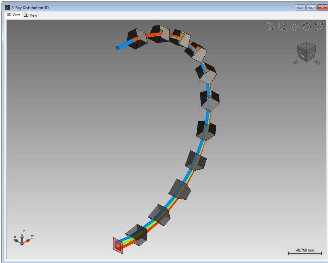
Zemax OpticStudio® is a well-distributed ray tracing software. VirtualLab Fusion allows to import optical systems with full 3D position information and glasses from Zemax OpticStudio®. After the import, the structure data of the optical system will be shown either as single surfaces, or can be combined into components in VirtualLab Fusion. One can perform ray tracing simulation of the imported optical system, and more importantly, field tracing could be performed to further analyze the system.
